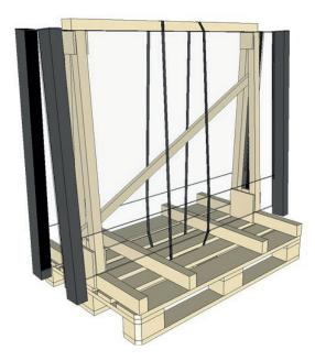
Each section is individually secured on the packaging to prevent ClickitUp® from falling during unloading.
